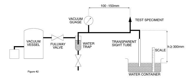
h: vertical distance between the edge at the inlet of the device and the water level.
