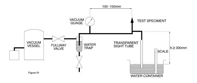
h : distance between the edge at the inlet of the device and the water level
