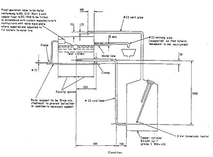
NOTE. Vent pipe to discharge 100 mm from sides of datern but not over float operated valve or float. If a lid is fitted cut a hole to permit any discharge, from the vent pipe, to enter the datern.
